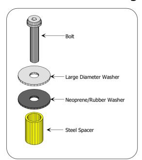
The principal with this fixing idea is basically the same whether you are using bolts or screws to fix your HDPE panels to either metal or timber frames or posts.
